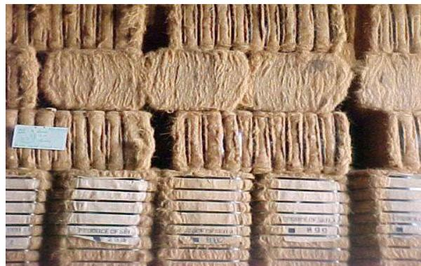
The cleaned fiber is screened, spread out in the mill yard to dry, picked up, baled, and shipped. Next, the fiber is spun by hand or machine into yarn and twine. Some fiber is also twisted
